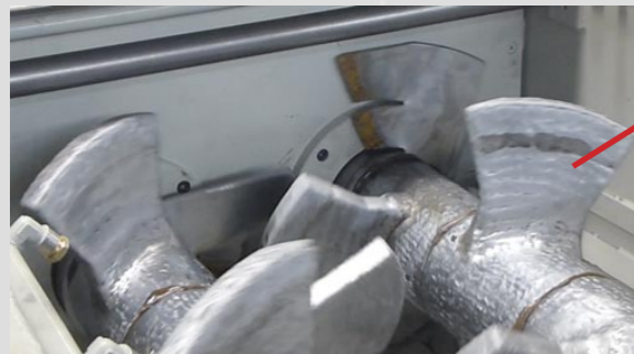
Scraper prevent clay residual at the rear wall
