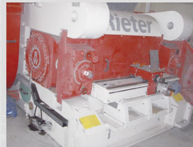
Switzerland – Fine roller mill
